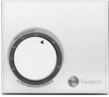
**MDEH1 Dehumidistat** - The wall mount dehumidistat monitors the humidity level in the area it is installed. When the humidity level rises above the desired set-point, the HRV will activate to high speed/override mode. Once the humidity level returns to desired condition, the unit will return to the normal mode. Typically used during heating season.
