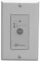
**RTS3 Pushbutton Timer** - This intermittent timer is the ideal control for those areas of the home where excess moisture, steam and odors are created. Press the button once to energize your HRV system to high speed for 20 minutes (green). Press the button twice and the unit will run for 40 minutes at high speed (yellow). Press the button three times and the unit kicks to high speed for 60 minutes (red). When time expires the unit will return to its original setting.
