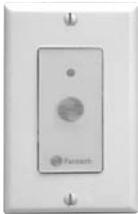
**RTS2 Pushbutton Timer** - The 20-minute remote timer is typically installed in areas where contaminated such as moisture and odors, are produced. Simply push the button and the HRV will activate to high speed for 20 minutes. Up to 5 electronic timers can be installed throughout the building at a distance of up to 500 feet (152 meters) from the HRV.
