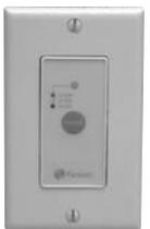
**EDF1 Triple Function Wall Control**- Triple-Function Wall Control makes it easy to control your home's indoor air quality system. Press the button once to run your HRV at a continuous low speed (green). Press the button twice and the unit will run 20 minutes on/40 minutes off (yellow). The cycle repeats continuously. Push the button three times and the system will run continuously on high speed (red).
